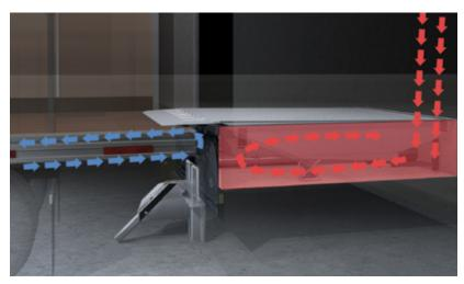
With PitMaster and optional Lip Corner Seals: Air trapped by the PitMaster Seal creates a pocket of "dead air" in the leveler pit, which acts as a thermal insulator that reduces heat transfer.
